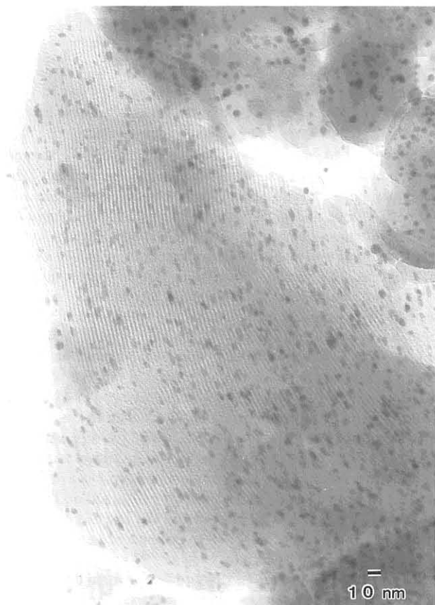
Figure 1. TEM photographs of 4.2wt.% Au/MCM-41 prepared by CVD and calcined in air at 673K for 4 hours.
